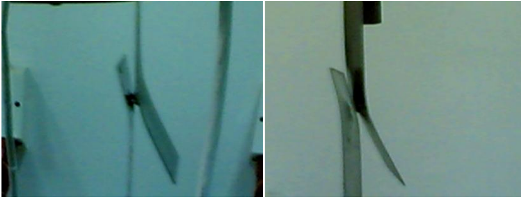
Fig. 3: Tensile shear test for the resistance spot-welded joint.
