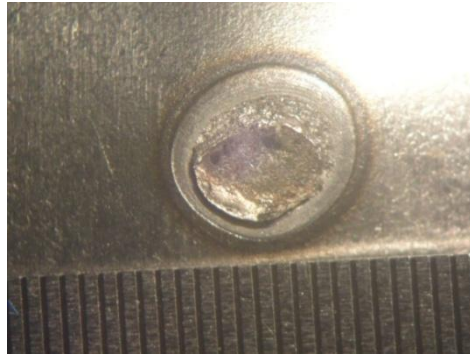
Fig. 14: Failure mode of spot dissimilar welded joint.
